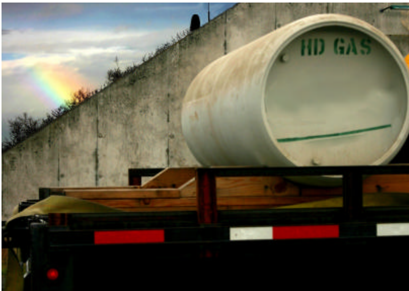
A bulk container of mustard agent is loaded on a truck outside a storage igloo as it is prepared for transport to the disposal facility. While marked as "gas," chemical agents are actually liquid in storage. Detonation would render the liquid into gas.
